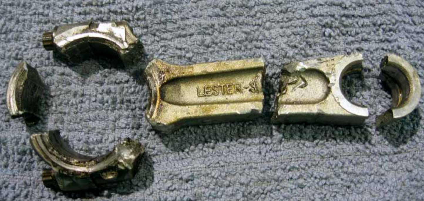
The connecting rod that blew the hole in the compressor case, shown on page 12.
