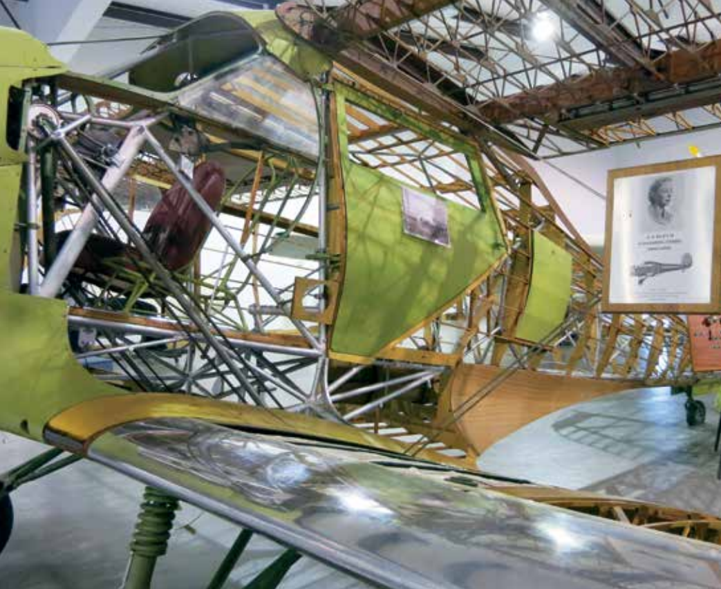
Known as the Olive Ann Beech Staggerwing exhibit, this 1938 E17B is displayed without its fabric covering so visitors at the Beechcraft Heritage Museum can see the intricate design details. Olive Ann donated the original 1933 engineering artifacts used for development of the Staggerwing's retractable landing gear.
