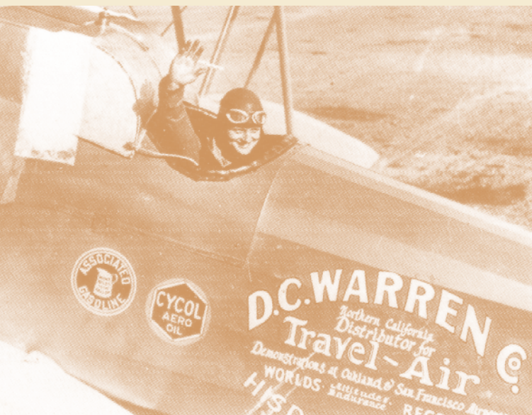
Known on the West Coast as an up and coming aviatrix, Thaden set a women's endurance record of 22 hours, three minutes, in March 1929, flying a Type 3000 equipped with additional fuel and oil tanks. The fuel tank mounted forward of the cockpit was crudely faired with sheet metal. The fuel line was routed into the cockpit where a wobble pump fed the gasoline to the fuselage tank. (EDWARD H. PHILLIPS COLLECTION)
