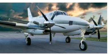
According to flight test data, BLR's certified five-blade, carbon fiber Whisper Prop provides between a 30 and 50 percent reduction in noise measured in dba, as well as some performance gains.
