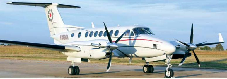
Commuter Air Technology's 350ME gives carrying capacity and endurance upgrades to the King Air B300 through two supplemental type certificates—one that increases operational gross weight and the other provides a fuel tank with the largest capacity of fuel in the market, adding a total of 280 gallons.
