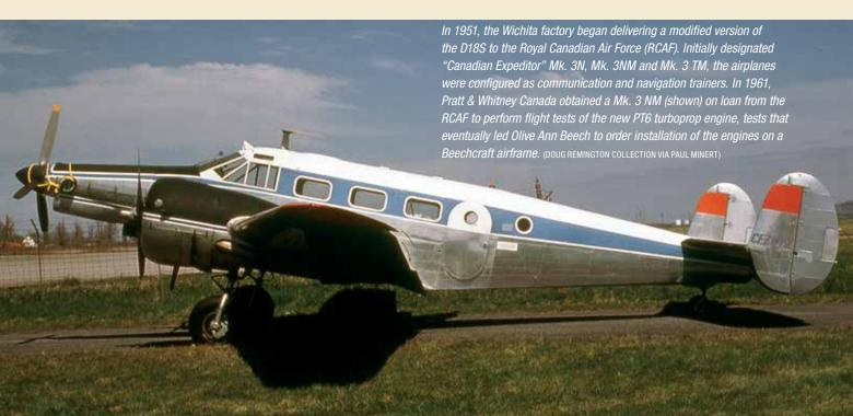
a better view of the sky and the earth below. Pratt & Whitney R-985 engines turning three-blade Hartzell constant-speed propellers was a feature of the G18S. A total of 154 airplanes were built from 1959-1963 when the final version of the venerable Model 18 took to the air.
