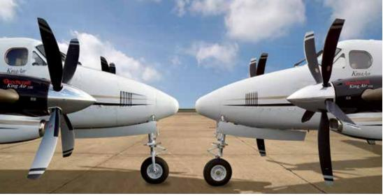
Raisbeck Engineering is now taking orders on its newly designed King Air 350 swept-blade propellers manufactured by Hartzell Propeller. The four-blade aluminum propellers and five-blade structural composite propellers have completed FAA certification flight tests and documentation, with STCs expected soon. According to the companies, the propellers offer increased across-the-board performance, lower cockpit and cabin sound levels and a striking ramp presence.
