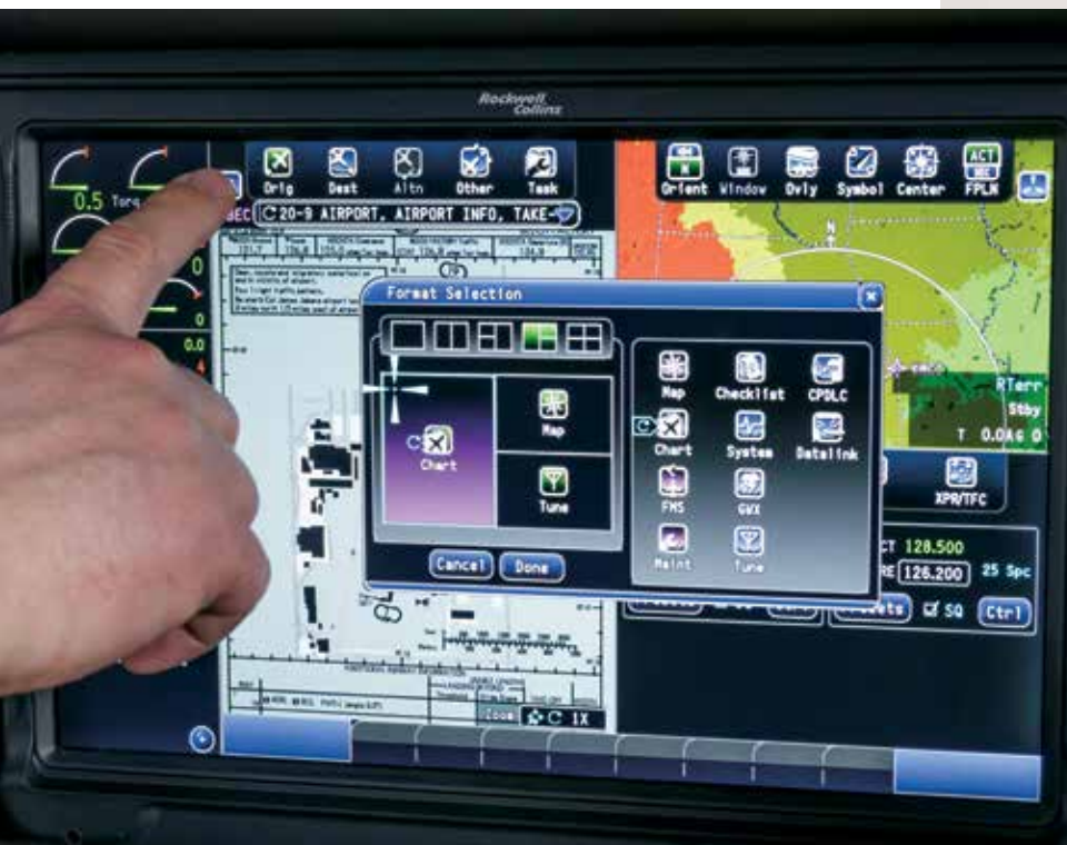
The touchscreens bring pilots intuitive interactive maps, easy-to-use icons, and the ability to simply touch the items that they want to control.
