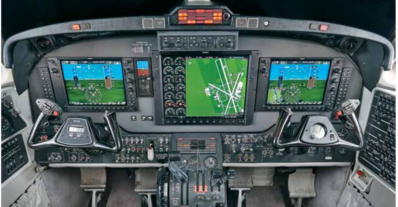
Garmin's integrated avionics system, the G1000.
