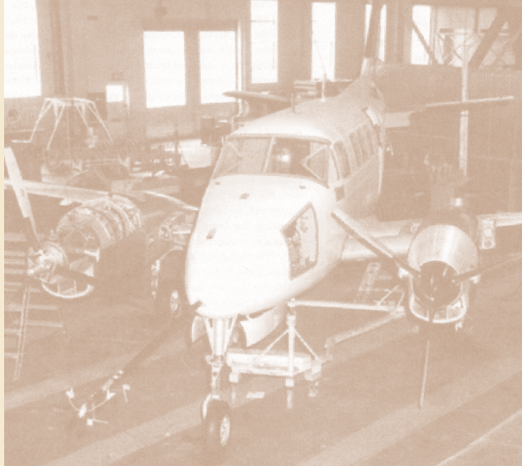
A Model 65 Queen Air airframe was modified to accept PT6A-6 engines in a bid to attract an order from the United States Army for a turbine-powered version of the piston-powered L-23F already in service.
