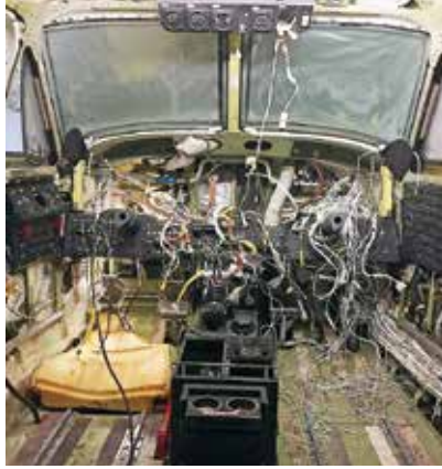
While undergoing its refurbishment, the panel and interior of the C90B was totally stripped down to metal and wires.
