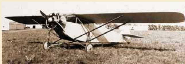
Clyde Cessna built a five-place monoplane in 1926 that would form the basis of the Travel Air Type 5000 cabin monoplane of 1927. Powered by one of Cessna's pre-war horde of Anzani radial engines, the ship's interior space could be converted into an air ambulance in a matter of minutes. Walter Beech flew the airplane and was impressed by its performance and handling qualities.
