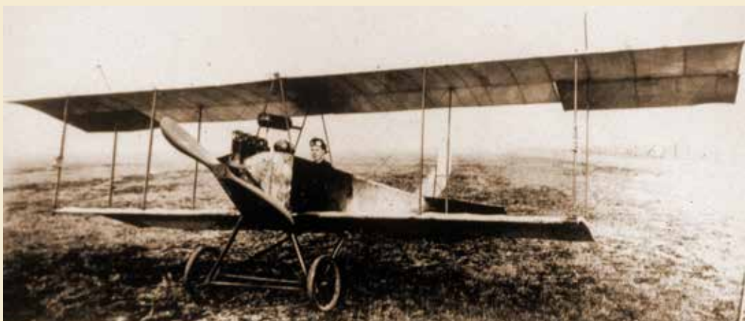
Laird with the " Boneshaker " biplane that he used for aerial exhibitions. Built in 1916, the airplane was his third design and was powered by an Anzani radial engine rated at 45 horsepower.
