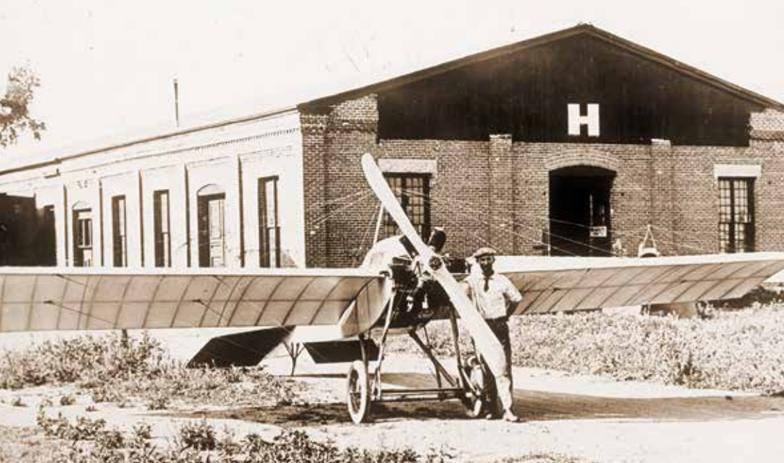
Clyde Cessna's best pre-war design was the two-place "Comet," powered by a six-cylinder Anzani radial engine rated at 60 horsepower. In 1917, Cessna posed with the recently-completed monoplane in front of the Jones factory. All of his early designs incorporated wing warping for roll control. (EDWARD H. PHILLIPS COLLECTION)
