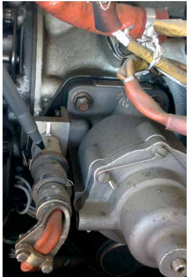
A pen pointing to the test solenoid of a King Air 200, with the overspeed governor directly to its right.
