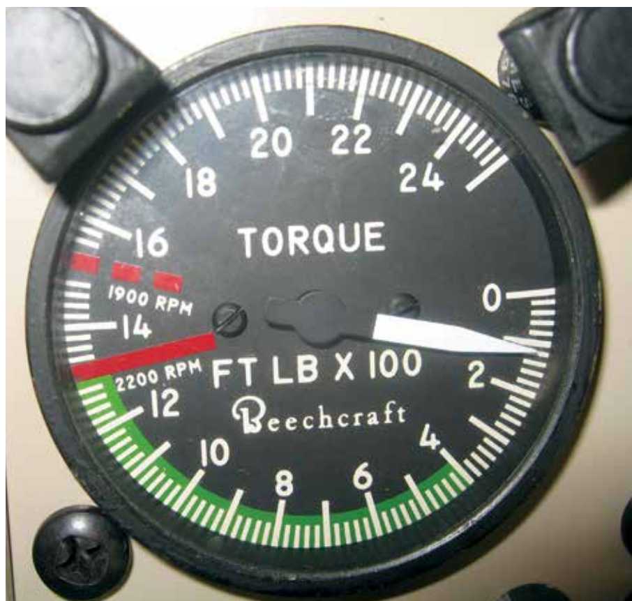
A torque gauge on a King Air E90 showing the limits in red.
