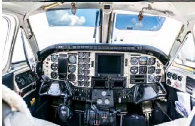
Hayot's upgraded panel with two GNS 430 WAAS, two Garmin transponders, a New Century autopilot and a new radar.
