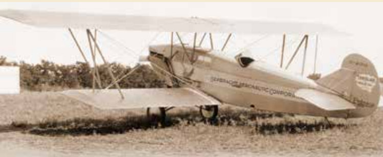
In 1925 Travel Air engineer Lloyd C. Stearman designed the Model BH cabin biplane powered by a 180-horsepower Wright-Hispano V-type engine. Four passengers could be accommodated in the cabin forward of the open cockpit. Featuring a wingspan of 42 feet, the Model BH was a large airplane and performed well, but only one was built. It was used by the Gerbracht Aeronautic Corporation. S-200 and Pegasus were not official designations used by Wichita's Travel Air Manufacturing Company. (EDWARD H. PHILLIPS COLLECTION)
