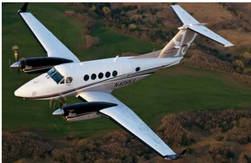
In 2011, composite curved propellers, winglets, and Raisbeck's Ram Air Recovery were added to the B200GT to make the new King Air 250.
