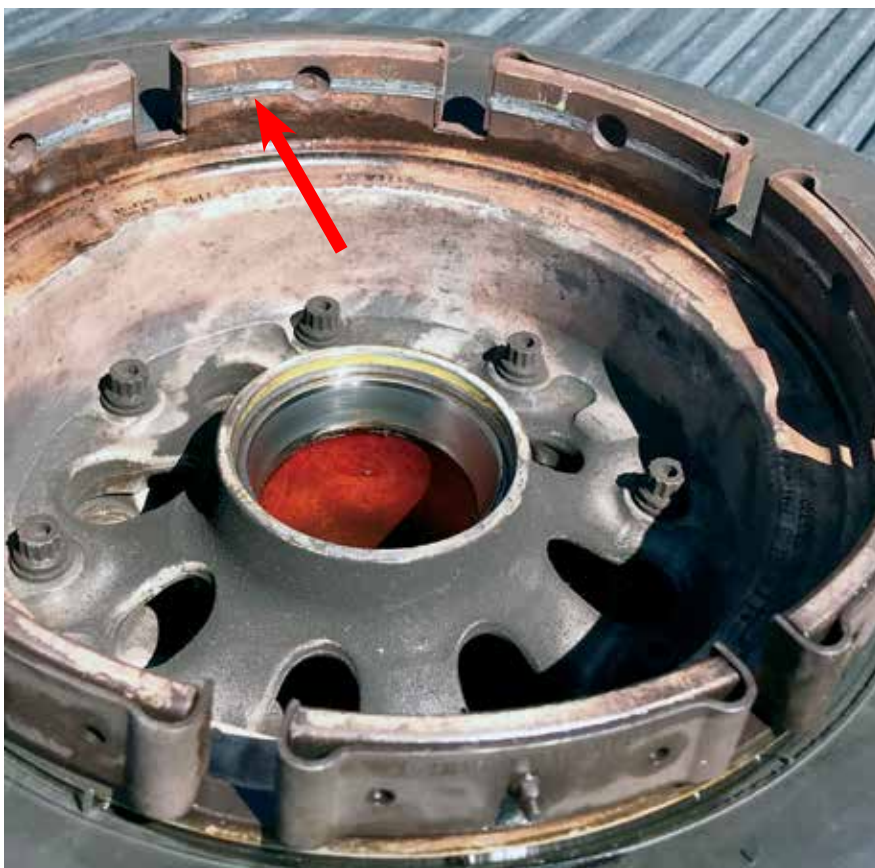
Photo G: Gouging on the wheel halves.
