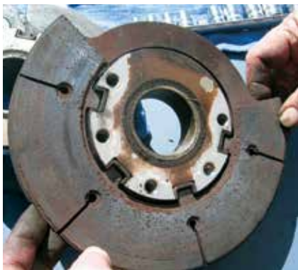
Photo B: The intact stationary disc. Notice the lugs fitting into receptacles in the brake caliper housing.
