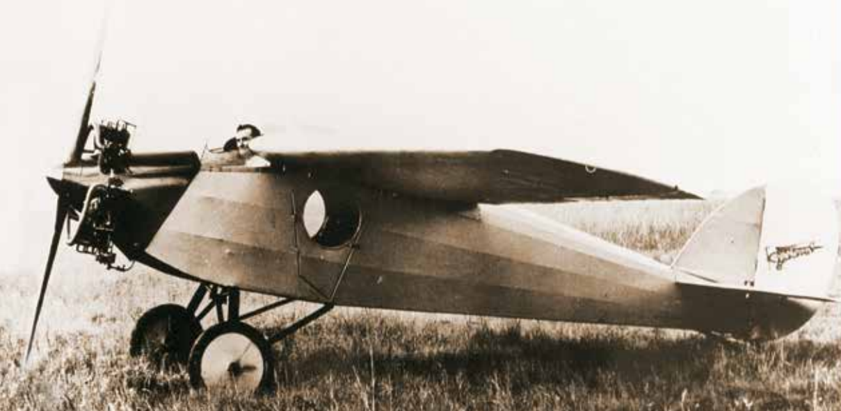
The "Phantom" was powered by the ubiquitous (but obsolete) Anzani radial engine, of which Cessna had acquired large numbers during recent years. The monoplane was first flown in August 1927 with local pilot Romer G. Weyant at the controls. (ROBERT PICKETT COLLECTION/TEXTRON AVIATION)
