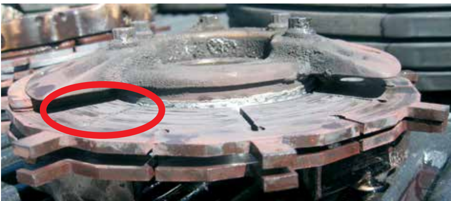
Photo E: The cooling slots in the rotating discs were filled with gunk, like the one circled above.
