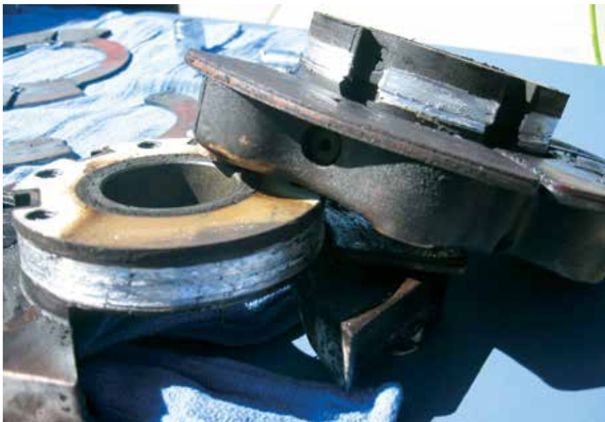
Photo F: Extreme gouging on the brake caliper housings, created by the stationary disc lugs once it broke into pieces.
