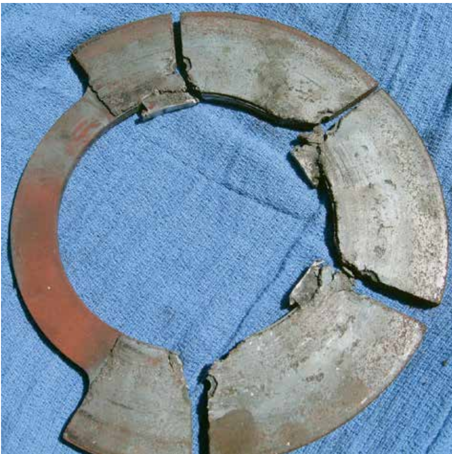
Photo C: One of the stationary discs pieced back together with what was left after the brakes were removed. Notice the three mangled lugs on the inside; one is missing completely.
