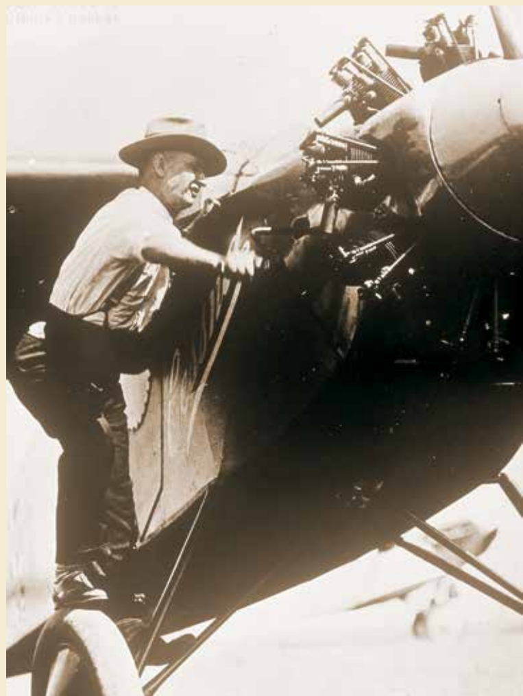
Clyde V. Cessna cranks the inertia starter on the Cessna-Roos Design No. 2, powered by a Wright J-4 static, air-cooled radial engine developing 200 horsepower. By 1929 sales of Cessna monoplanes were increasing, particularly the Model AW. (TEXTRON AVIATION)
