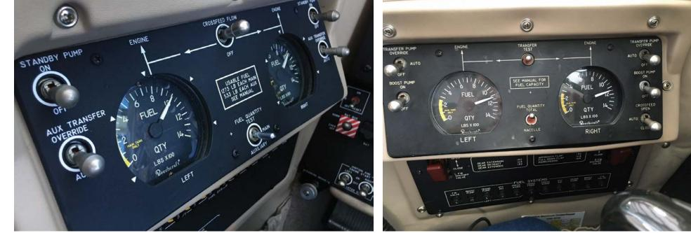
The fuel panels of the King Air 350 (Figure 7, left) and the C90A (Figure 8, center).
