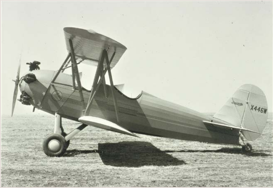
The CW-12K was powered by a Kinner B5 static, air-cooled radial engine rated at 125 horsepower. Travel Air Division engineers Herbert Rawdon and Ted Wells designed the CW-12 series airframe to accommodate four different engines ranging from 90 to 165 horsepower. Only two are known to have been built. (Edward H. Phillips Collection)
