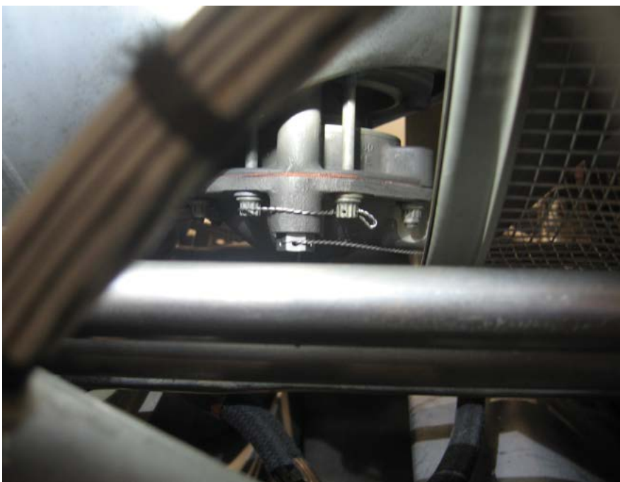
The bleed valve on a King Air C90's PT6A-21 engine in the 6 o'clock position. You can see part of the inlet screen to the right.
