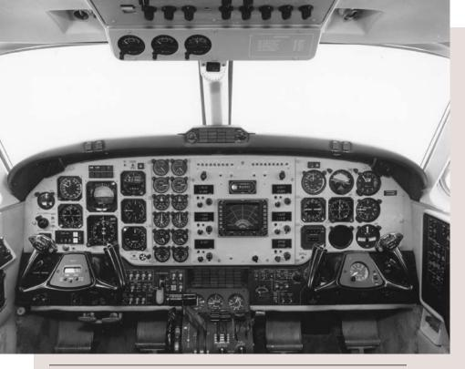
The Super King Air's flight deck was similar to those of its siblings but featured digital avionics, weather radar and autopilot/flight director. Overhead console housed ammeter, DC load meters and lighting rheostats; subpanels contained switches for primary and secondary airframe systems. (University Archives and Special Collections, Wichita State University Libraries)
