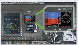
ThrustSense is commanded by the Standby Display Unit that is the pilot's interface mode for speed and torque selections.
