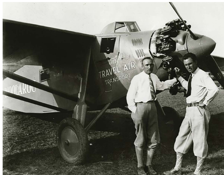
The “Woolaroc” was completed during the first week of August 1927. Note the cockpit cupola and sliding window; nine-cylinder Wright Aeronautical J5 static, air-cooled radial engine; exhaust collector ring and the Pioneer Instruments drift indicator mounted on the cockpit door.
