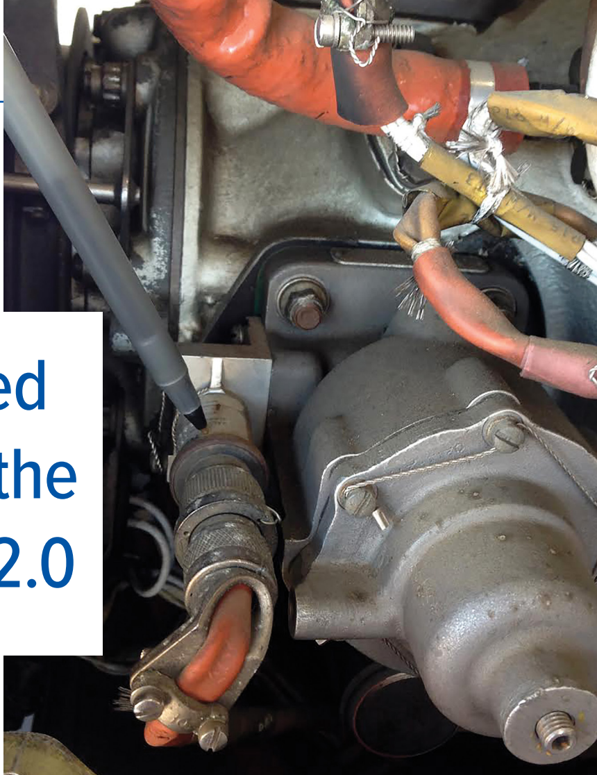
An overspeed governor on a King Air B200, with the solenoid pointed out (at left).
