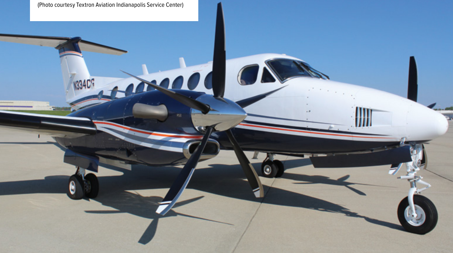
Among the laundry list of upgrades Giles made to FL-586, installing Blackhawk Pratt & Whitney Canada PT6A-67A engines and 5-blade propellers has been among the most noticeable – from improved climb rate to jet-like speed and a quieter cabin. (Photo courtesy Textron Aviation Indianapolis Service Center)
