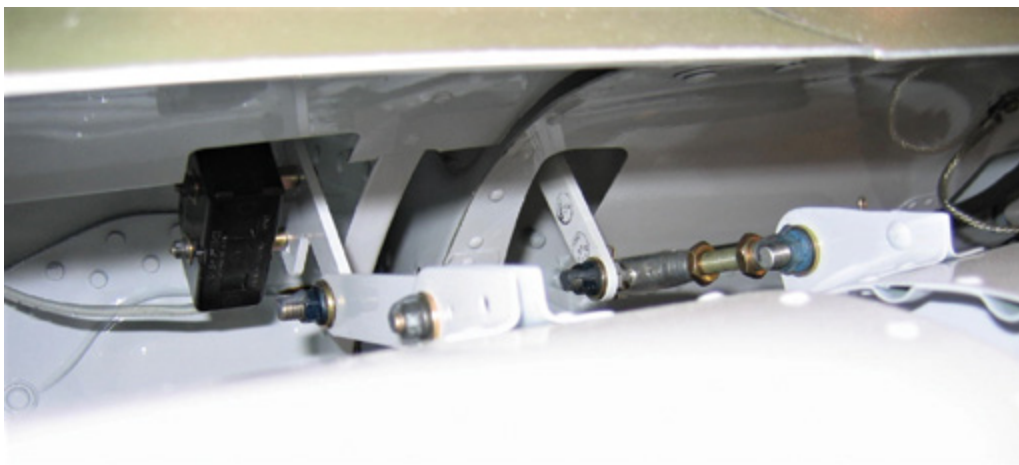
The Split Flap Protection switch and its connections to both inboard and outboard flap segments.
