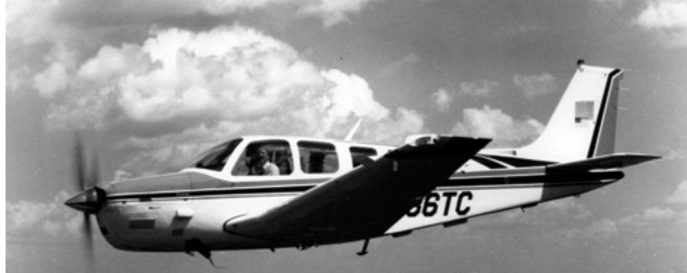
Introduced in 1981, the B36TC featured significant upgrades that set it apart from its predecessor, the A36TC. An important improvement was the airplane's fuel capacity that was increased to 108 gallons. Production was terminated in 2002 after 424 airplanes had been built. (Wichita State University Libraries, Special Collections and University Archives)
