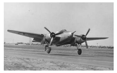
The Model 28 Destroyer would have lived up to its name had it been deployed to the Pacific Theater of War in 1945. The nose-mounted 75 mm cannon could fire up to 20 rounds of various high explosives and the twin 0.50-caliber machine guns would have further multiplied the XA-38's impressive firepower. (Courtesy Beechcraft Corporation, Special Collections and University Archives, Wichita State University Libraries)
