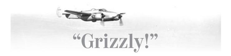
In 1945, Beech Aircraft Corporation built the most powerful ground attack aircraft of World War II – the mighty XA-38 Grizzly. Armed with a 75-mm cannon and six machine guns, the twin-engine gunship was large, powerful and fast, but the war ended before the enemy could feel its offensive punch.
