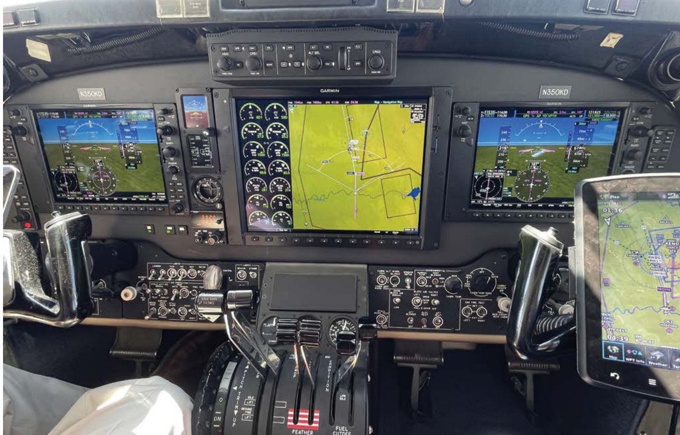
One of Daniel Herr's first upgrades after purchasing FL-136 in 2017 was to Garmin G1000 NXi avionics optimized by Stevens Aviation. (Credit: MeLinda Schnyder)
