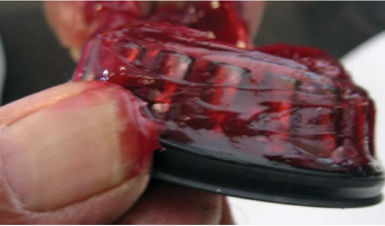
Figure 3: Wheel bearing packed with grease and ready for reinstallation.
