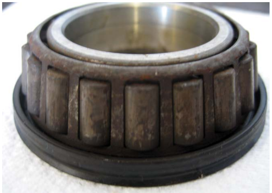
Figure 1: The totally dry wheel bearing, taken from the King Air referenced in the article.
