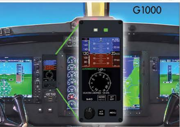
Standby Display Unit serves as pilot's interface
