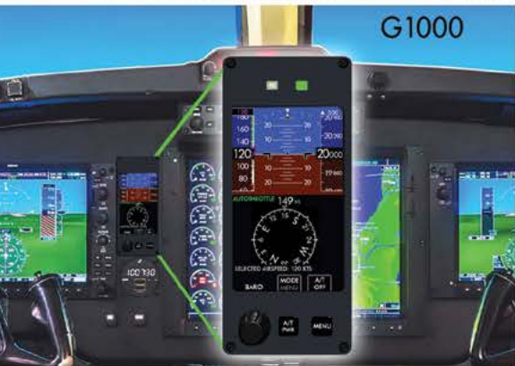
Standby Display Unit serves as pilot's interface
