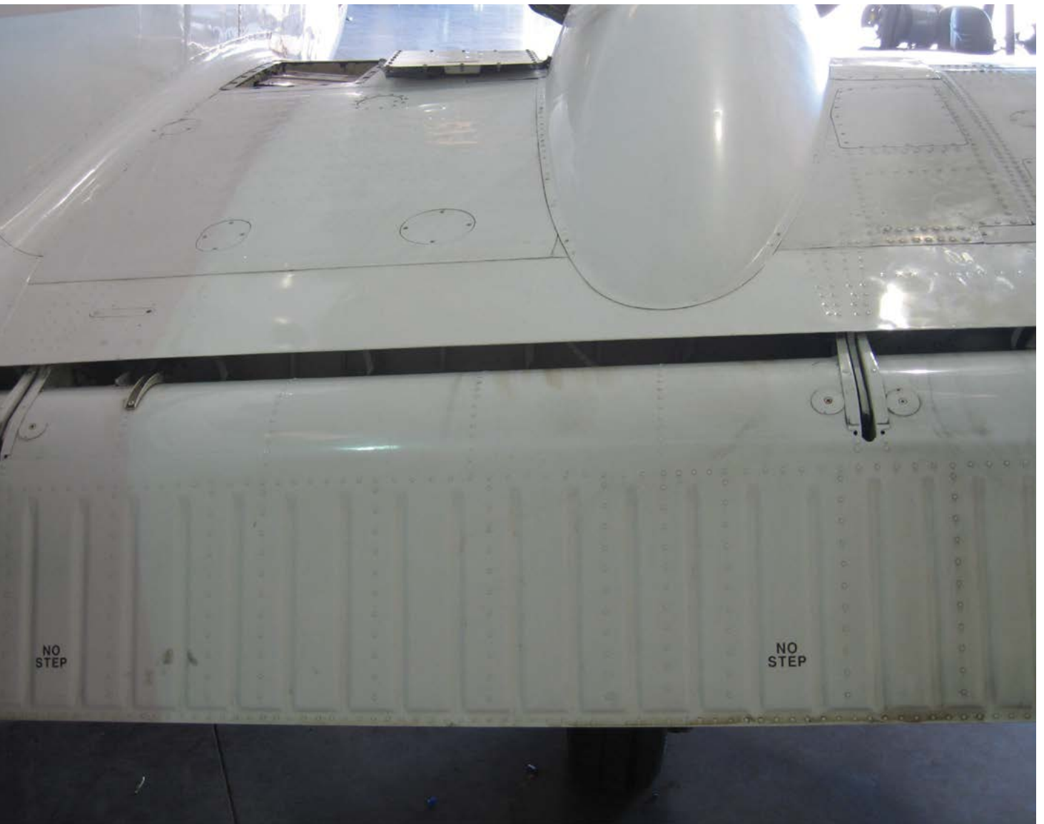
Figure 2: The wing flap in the down position is how you can check the flap track assemblies; they flank the central area of the flap as viewed from the trailing edge.
