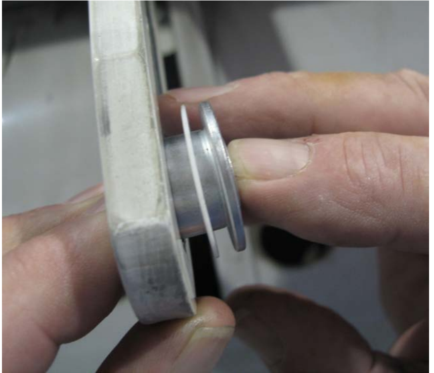
Figure 1: A close-up of the washer and roller bearing installed on the flap track assemblies. The Teflon washer is thin and white, and it's positioned under the thicker silver roller bearing.
