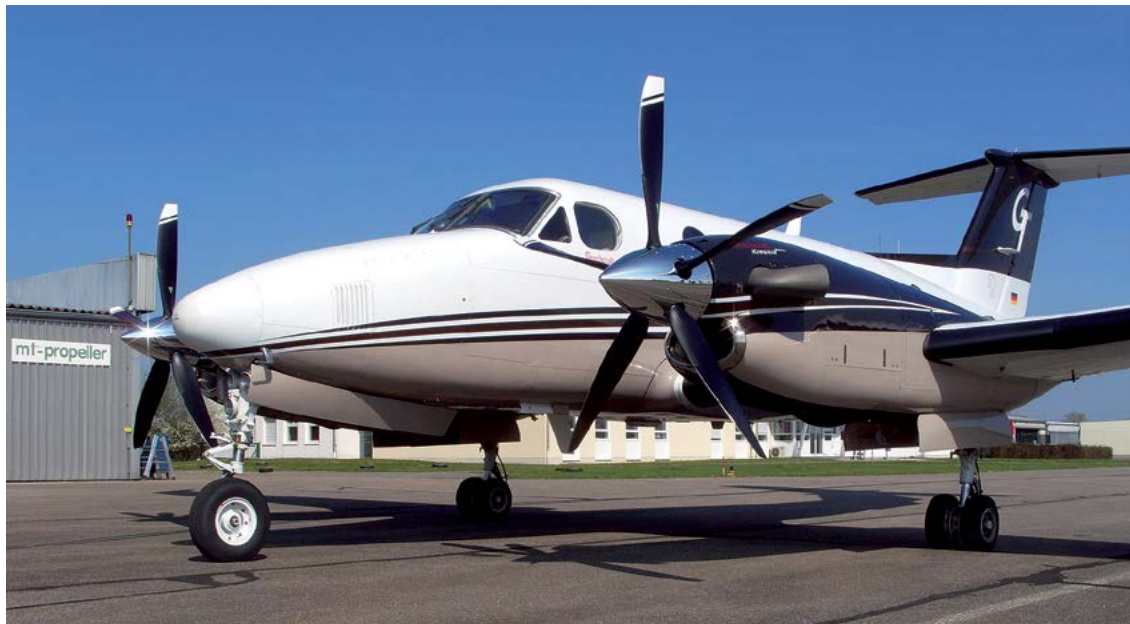
MT-Propeller's five-bladed Quiet Fan Jet composite prop.
