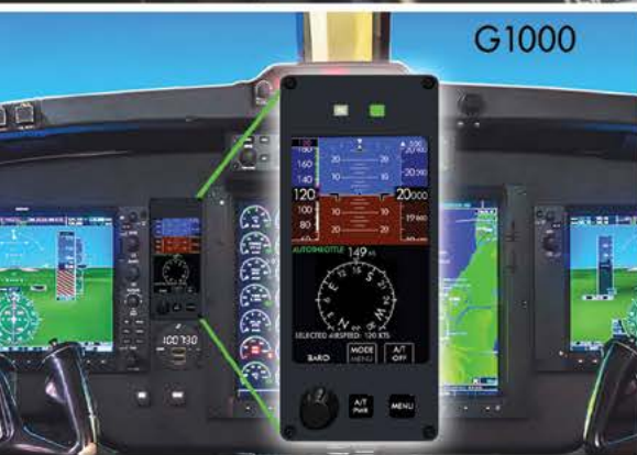
Standby Display Unit serves as pilot's interface
