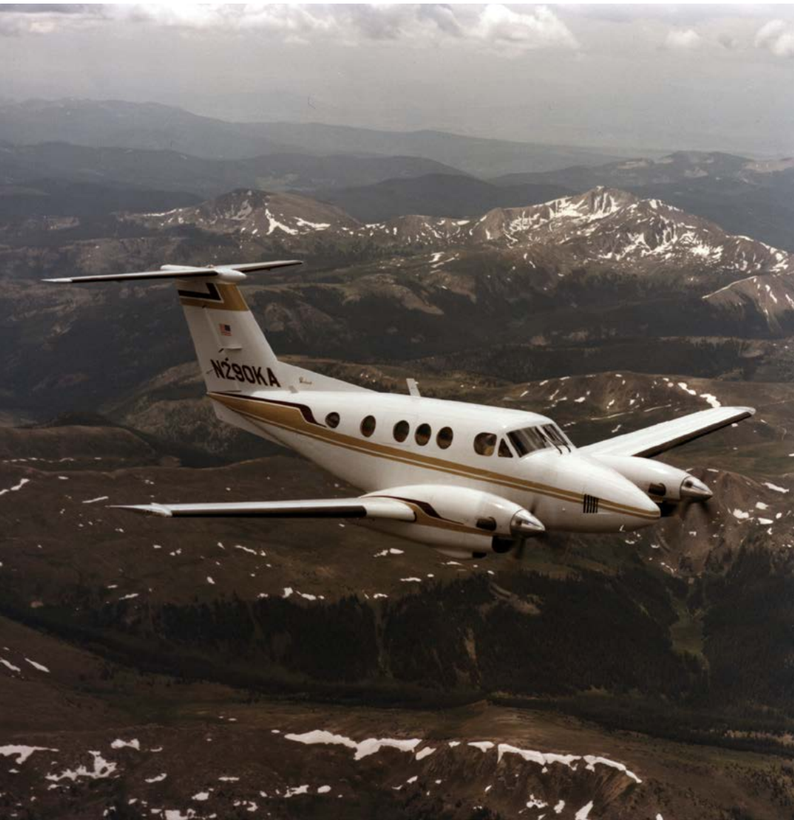
Beech Aircraft Corporation capitalized on the advantages of the Model 200 Super King Air's T-tail arrangement by applying it to the F90 and F90-1. (Special Collections and University Archives, Wichita State University Libraries)
