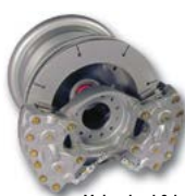
Main wheel & brake Kit P/N 199-90
