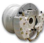
Main wheel & brake Kit P/N 199-110
