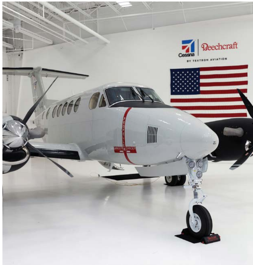
Beechcraft King Air 260 Multi-Engine Training System (METS) T-54A for the U.S. Navy.
