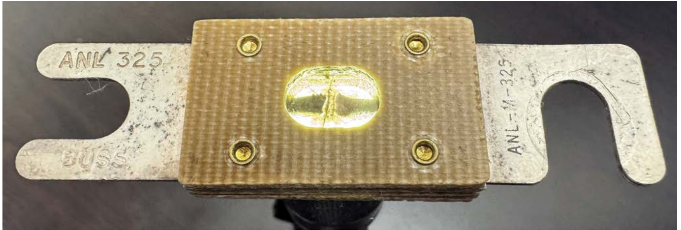
A failed 325a current limiter
