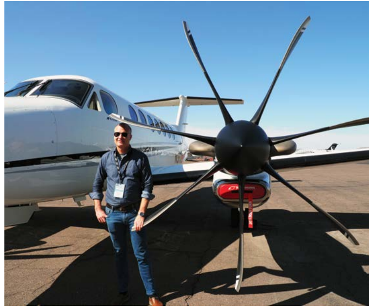
MT-Propeller Vice President Martin Albrecht was at King Air Gathering in March with the recently certified 7-blade Whisper Prop installed on a King Air 350 also featuring Blackhawk's XP67A Engine+ Upgrade.
