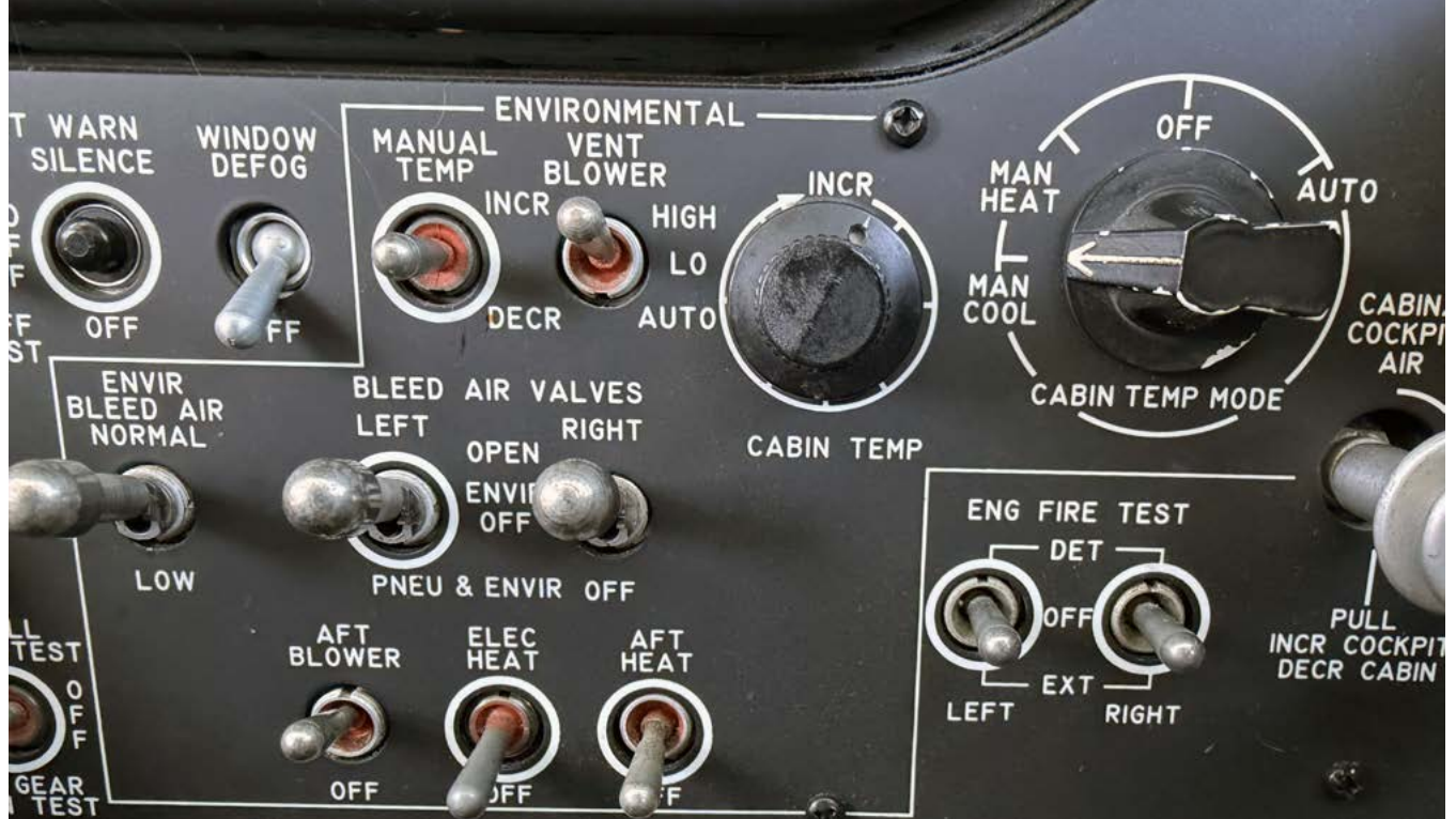
A look at the King Air's environmental system panel.
