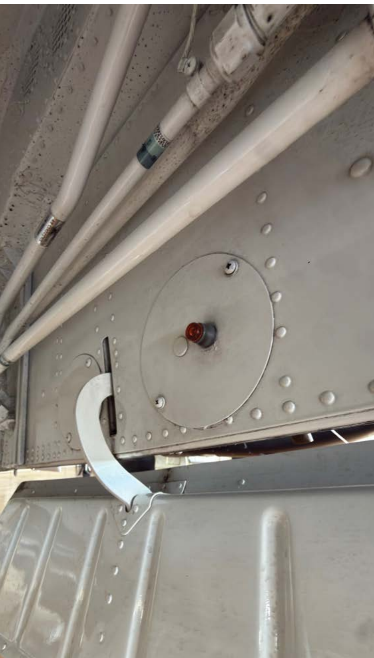
If you fly a King Air 3XX, the reset switch in the front wheel well should be a part of every preflight.
