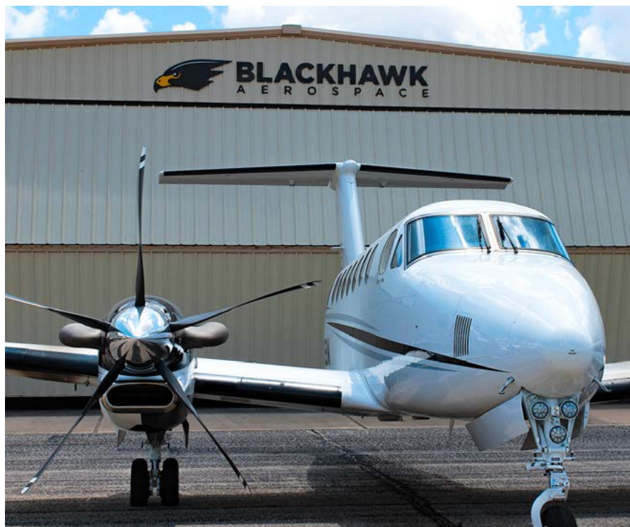
The FAA approved Blackhawk’s STC to integrate Hartzell 5-blade composite propellers on its King Air 350 XP67A Engine+ upgrade.
