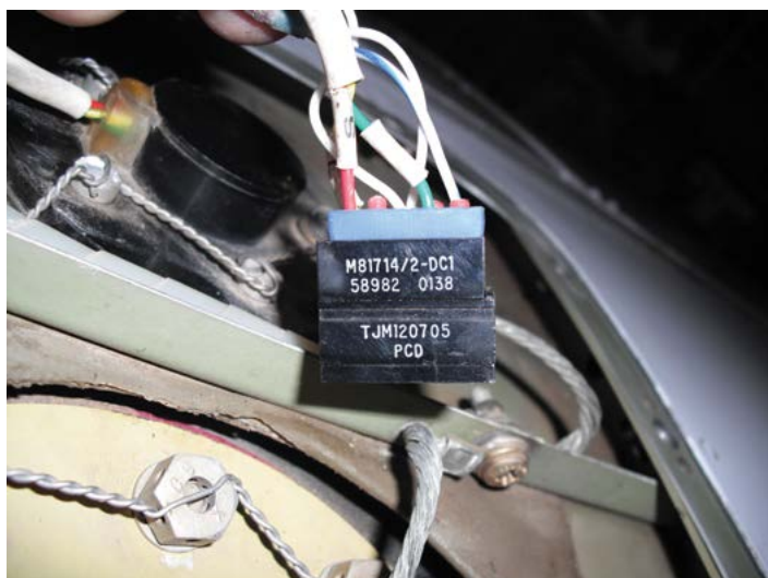
Operators can improve the reliability of their systems by changing one matrix block to three 4-way splices.
