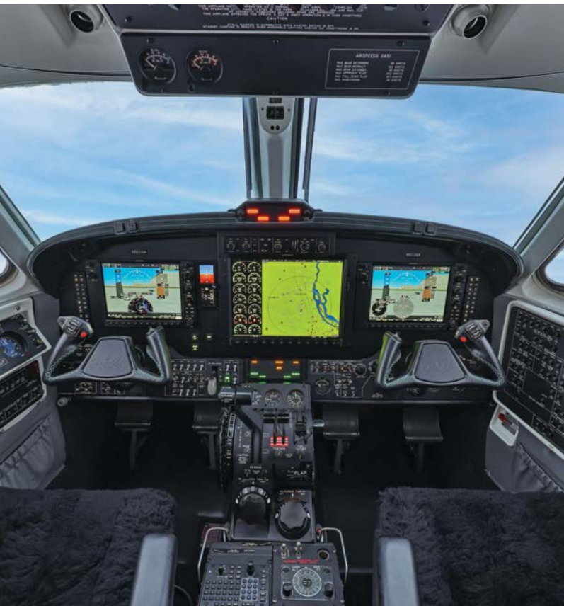
The Herrings upgraded BB-1462 to Garmin G1000 NXi avionics with Autothrottle and Autoland. Custom yokes match the contrasting teal stitching on black leather found in the cabin.
