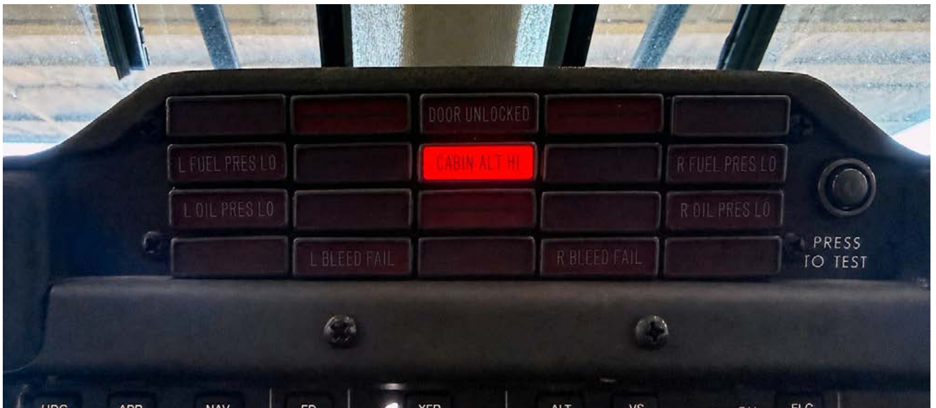
In more modern King Air models, there is a secondary CABIN ALT HI red warning light, which presents on your caution/advisory/warning panel when your cabin exceeds 12,500 feet.
