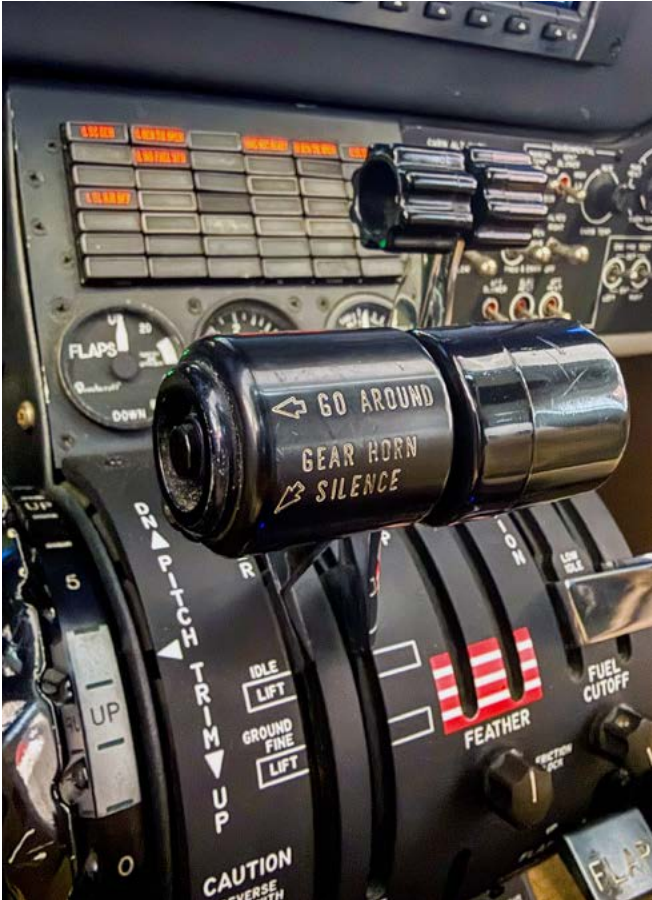
In most King Air models, there is a way to mute the gear warning.
