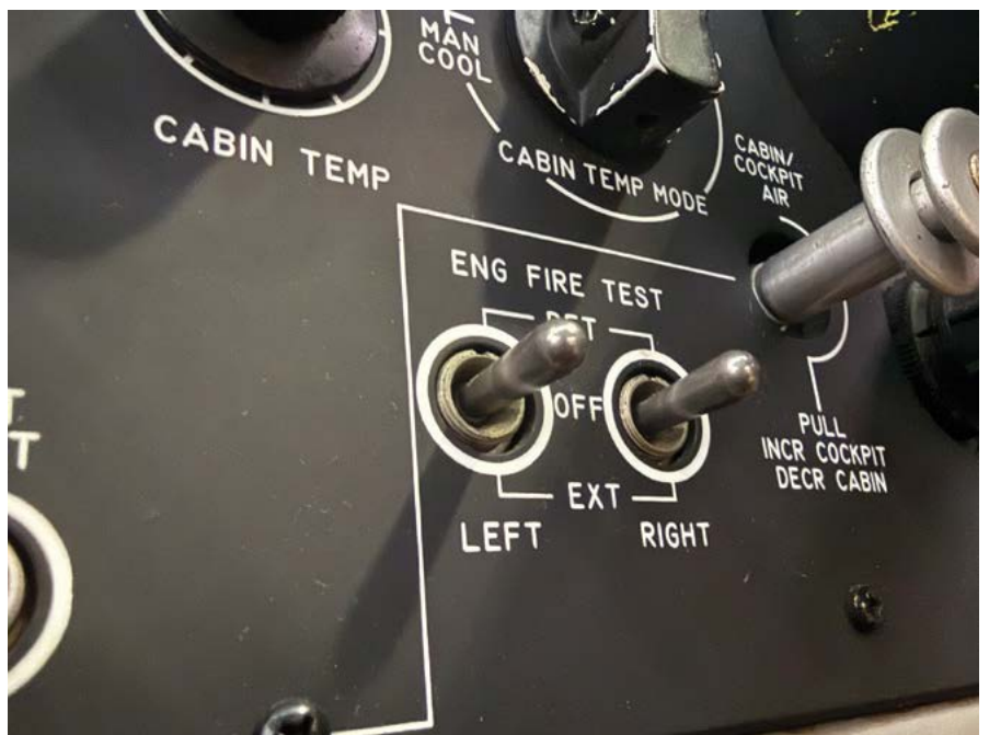
Fire Extinguisher Test switch
