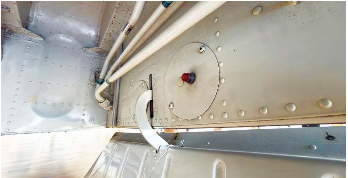
Joe would address concerns with the King Air's cooling system, including relocating the compressor reset for King Air 3XX models from the nose gear bay.
