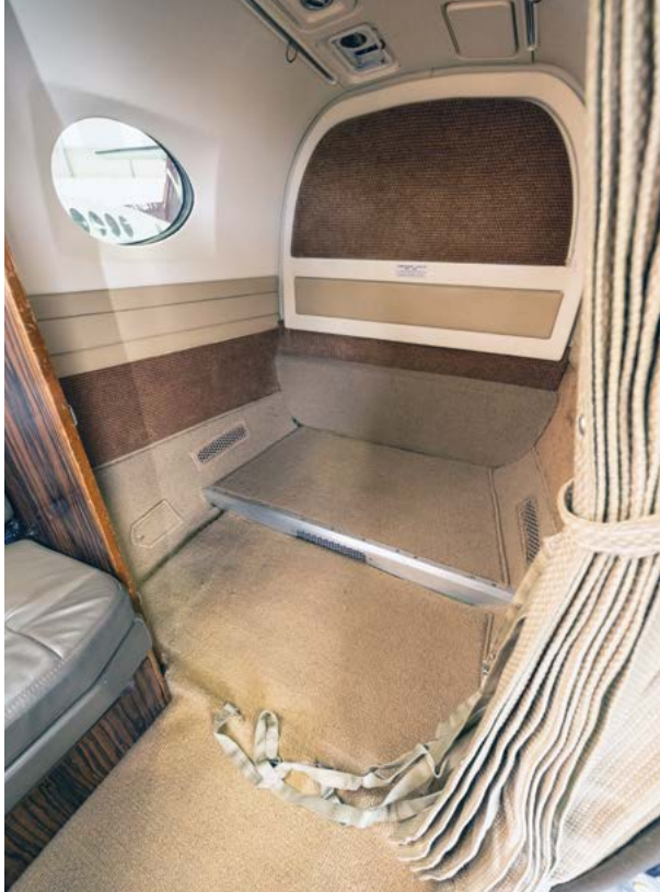
Loading and unloading could be so much easier if the King Air's cargo space had a flat floor. Some owners have developed their own solutions like this plywood platform.
