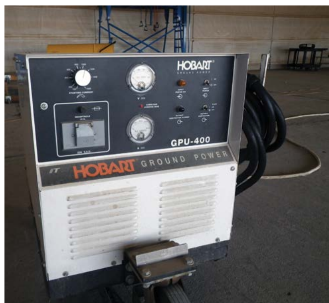
There are many power carts that will meet the starting voltage and current requirements for a King Air.
