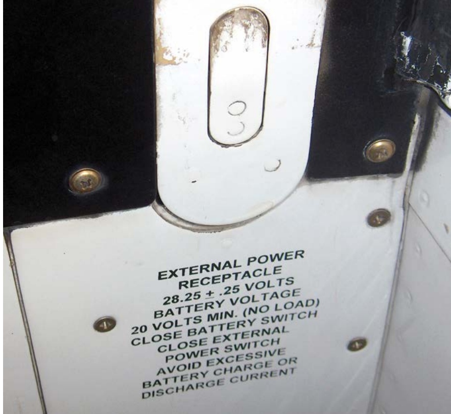
A common concept is: Do not connect external power when the aircraft battery is below approximately 20 volts.
