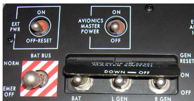
All models recommend (or in some cases require) the battery switch to ON.
