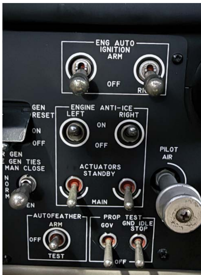
The engine anti-ice switch moves the ice deflector in the front of the engine and opens the door behind the engine where debris can be ported overboard.
